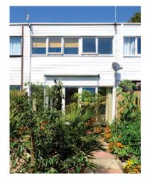
For a relatively modest build cost of £70,000, a smart modern home has been created, with extraordinarily low carbon emissions. The south facing glazed screen wall enables excellent solar gain and the effective and well detailed insulation means gas bills are only £27/month and electricity is £23/month. As the roof mounted solar PV are producing an income of over £600 pa, the house is close to being both carbon neutral and energy cost neutral.
